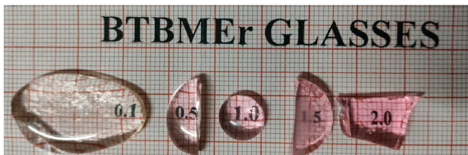
Fig. 1. The photograph of different concentration of Er-doped borotellurite glasses.
